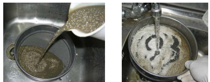
Figure 6: Separation of the Ca-P recovery product from waste activated sludge after anaerobic treatment
