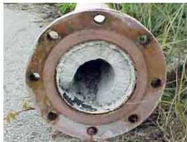
Figure 1: Struvite scalings in WWTP with enhanced biological phosphorus removal are a common operational problem
