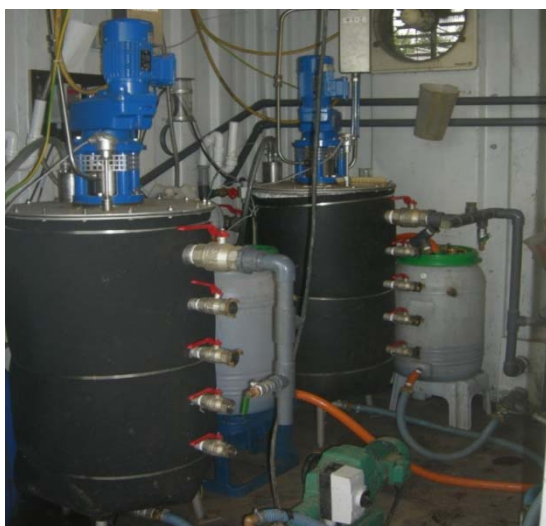
Figure 4: 150 L laboratory digesters that were used for the development of the FIX-Phos process
