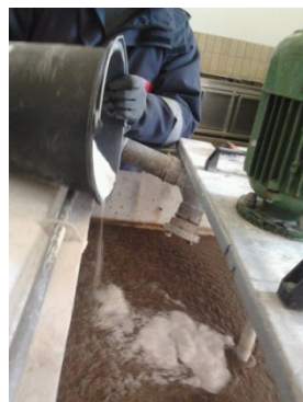
Figure 2: CSH is mixed with waste activated sludge during a full scale test before the CSH/sludge mixture is fed into the digester.
